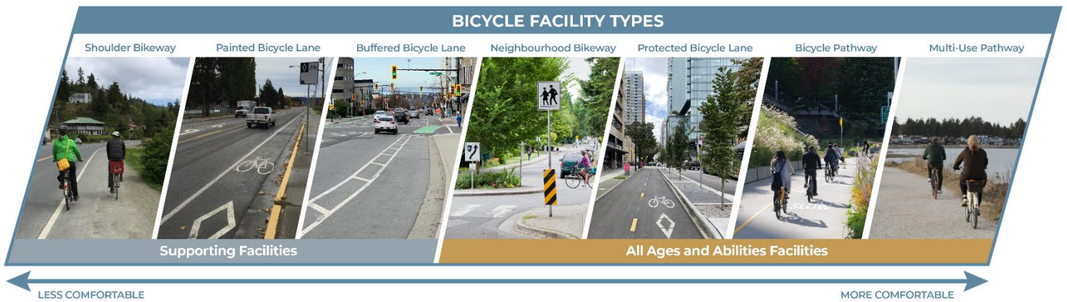
Figure 19: Bicycle Facility Types
